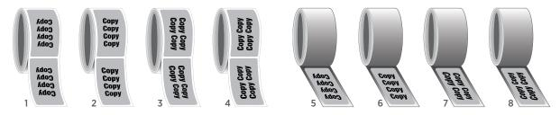
**Draw / Repeat:** Refers to the distance from the top edge of one label to the top edge of the next label. The length of the label plus the gap equals the repeat. **Length + Gap = Draw / Repeat**
